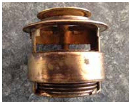
This is the other style thermostat note the sleeve is at the opposite end
