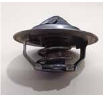
This is the incorrect type of thermostat for by pass radiator systems. It will not close off the recirculation circuit
